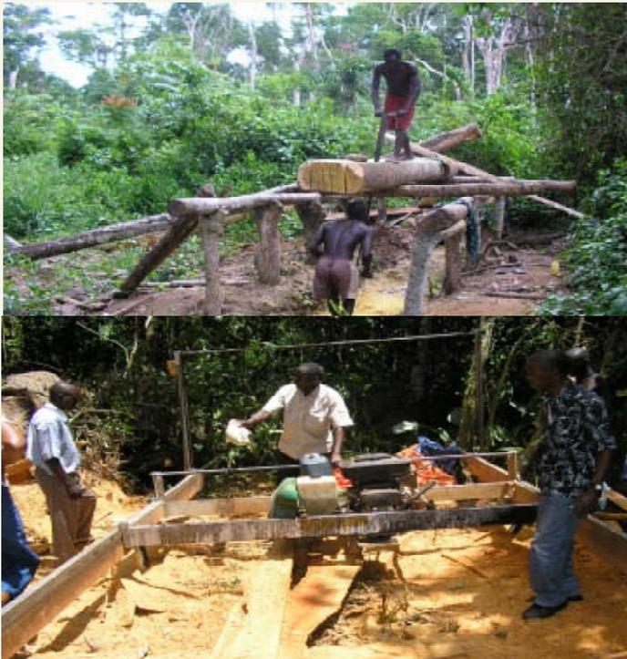
Figure 3.4: Top to Bottom: Lumberjacks manually converting a log and a private forest owner using a mobile saw mill to convert logs into timber. The mobile saw mill is more cost effective, efficient and profitable, thus the high value retained by the private owner as compared to the lumberjacks who use the traditional hand saw.
