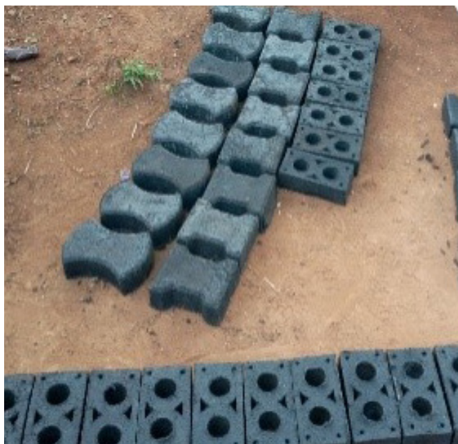
Samples of plastic waste recycled into stone pavers and ventilators by different youth groups selected to pilot the initiative in Rhino camp and Omugo extension in Arua
