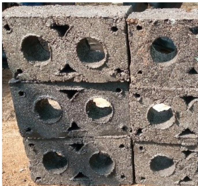
Samples of plastic waste recycled into stone pavers and ventilators by different youth groups selected to pilot the initiative in Rhino camp and Omugo extension in Arua
